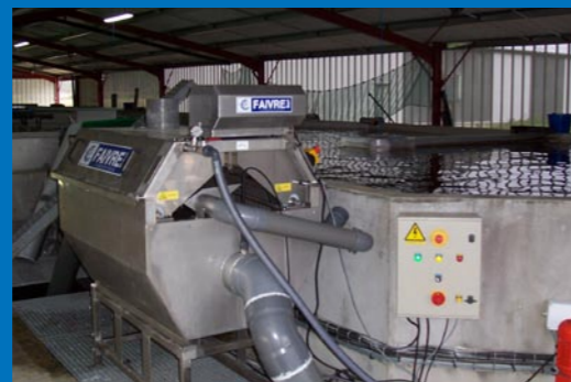
Model 4-80 with 36µ mesh on recirculation system.
