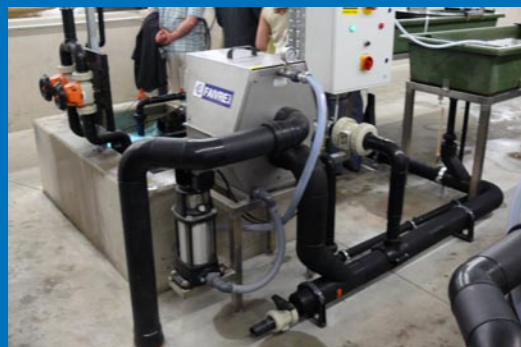
Model 2-40 with 36µ mesh on recirculation system.
