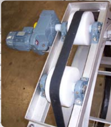
Simple and robust drum driving system.
