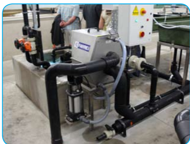
Drum filter model 1-40 with tank ( in sturgeon recirculation system )
