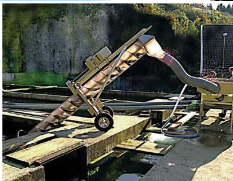
77 ALU CLASS Ø330 mm elevator working at land based trout farm.
