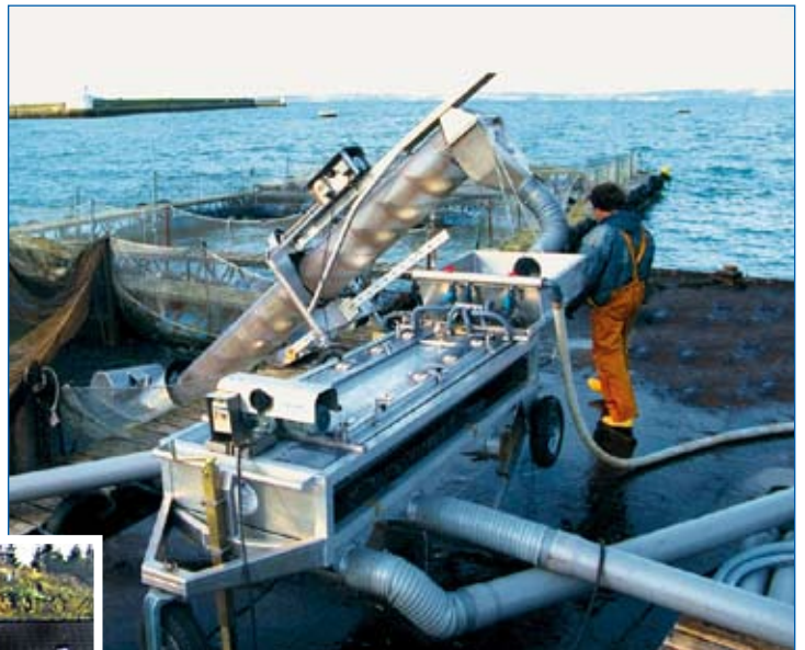
77 ALU CLASS Ø450 mm elevator working on sea cages.
