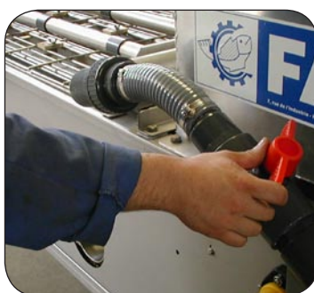
Water flow regulating with valves
