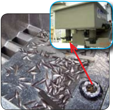
Inlet hopper with special system to plug a fish pump.
