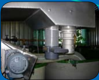
Motoreductor IP 55, with 3 speed by belt system.
