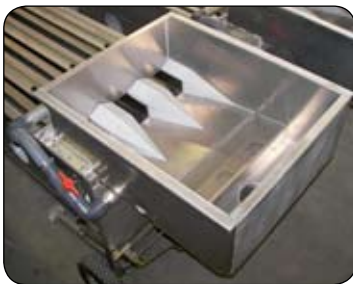
View inside the inlet hopper
