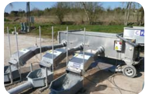
Helios 50 and 3 counters with reception tank.
