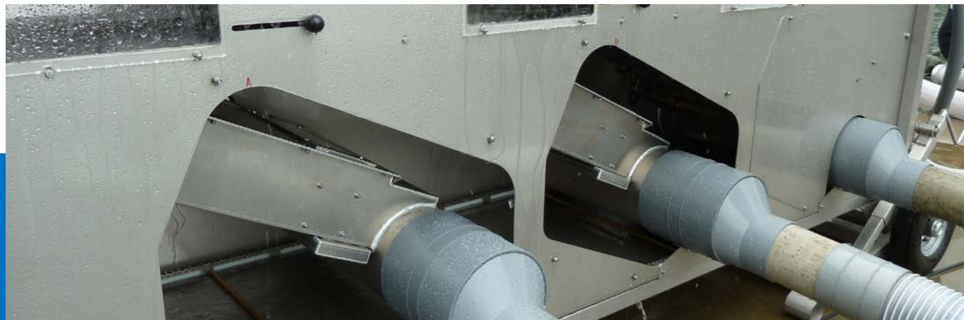
The Pescavision counters located inside the grader are easy to access.
