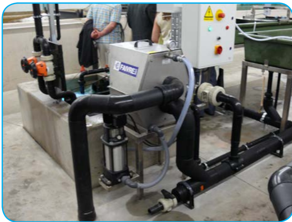
Drum filter model 1-40 with tank ( in sturgeon recirculation system )
