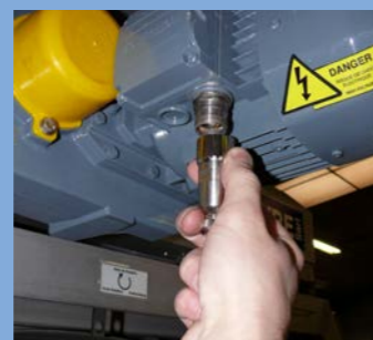
Model 4-80 with 36µ mesh on recirculation system.
