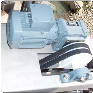
Drive and suspension of the drum by belts. (Simple and robust solution)
